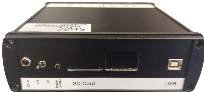
Figure 1.3: Logger front side with 12V-in, on/off switch, display switch, SD card slot, display and USB connector.
